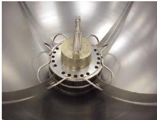
Figure 4: PMD for Horizontal Handling
