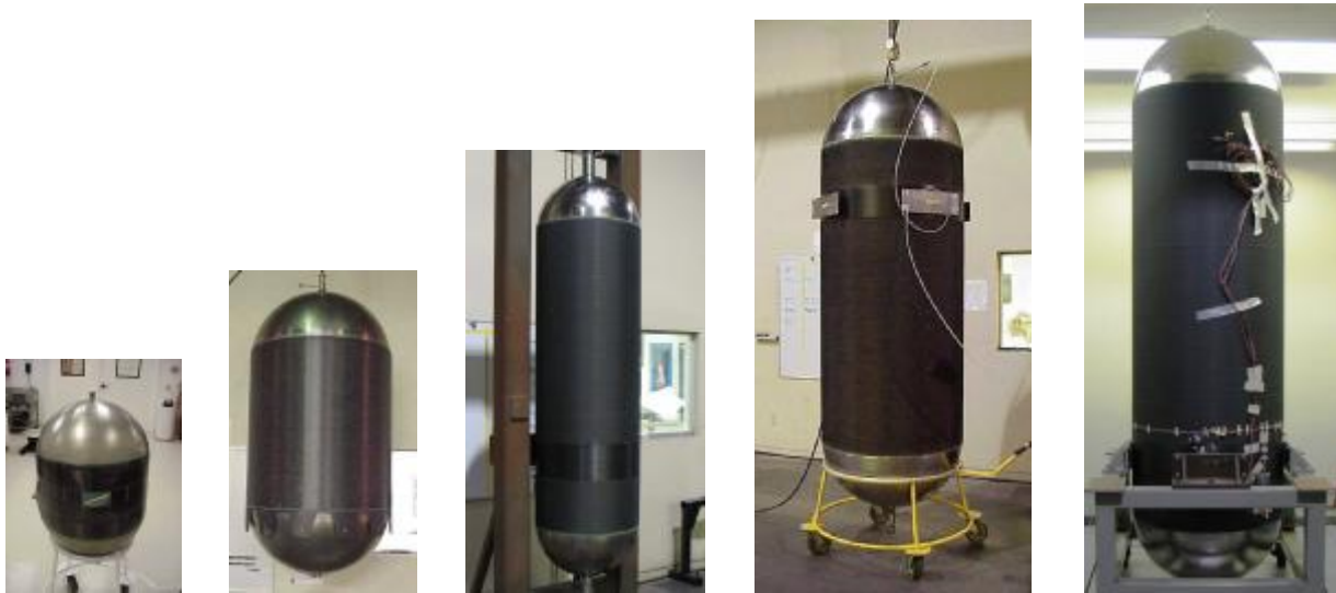
Figure 1: Hybrid Propellant Tanks
