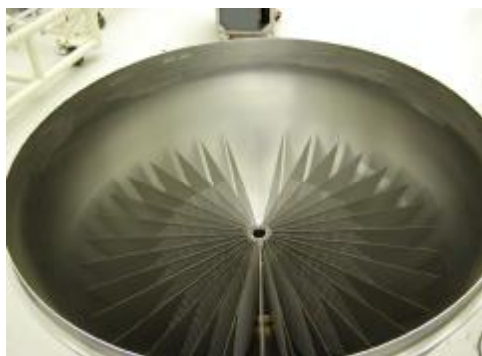
Figure 6, PMD Designed for Propellant Center-of-Mass Control
