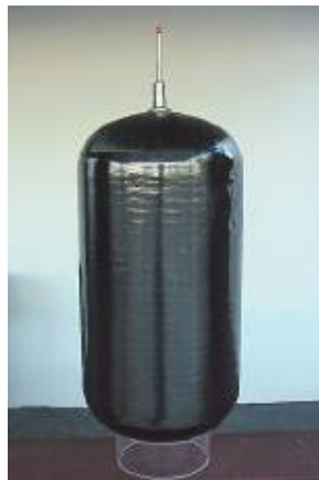
Figure 10: A completed VEGA Gas Tank
