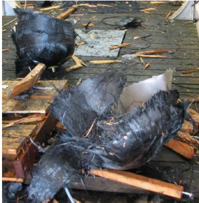
Figure 9: Qualification Tank After Burst
