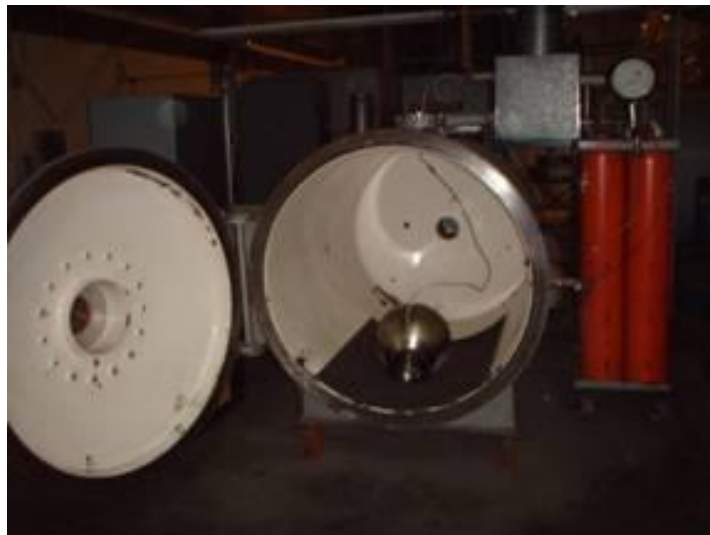
Figure 6: External Leak Testing Set-Up
