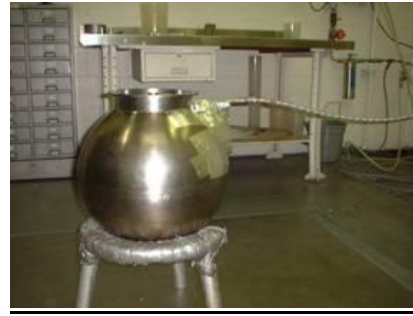
Figure 9: Pressure Testing Set-Up
