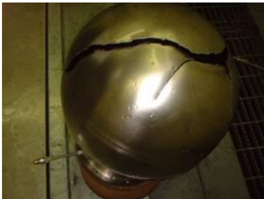
Figure 10: Qualified Burst Tank
