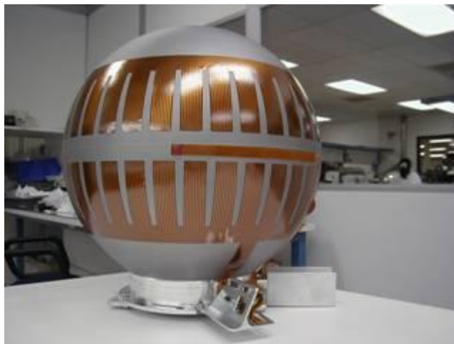
Figure 5: Pressurant Tank Assembly shown with heaters, sensors, cables and flight bracket installed.
